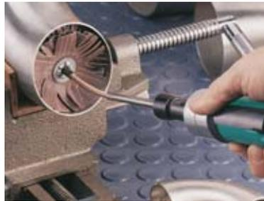
3" Eyelet Sanding Star easily enters pipe elbow using 7" long flexible mandrel.
