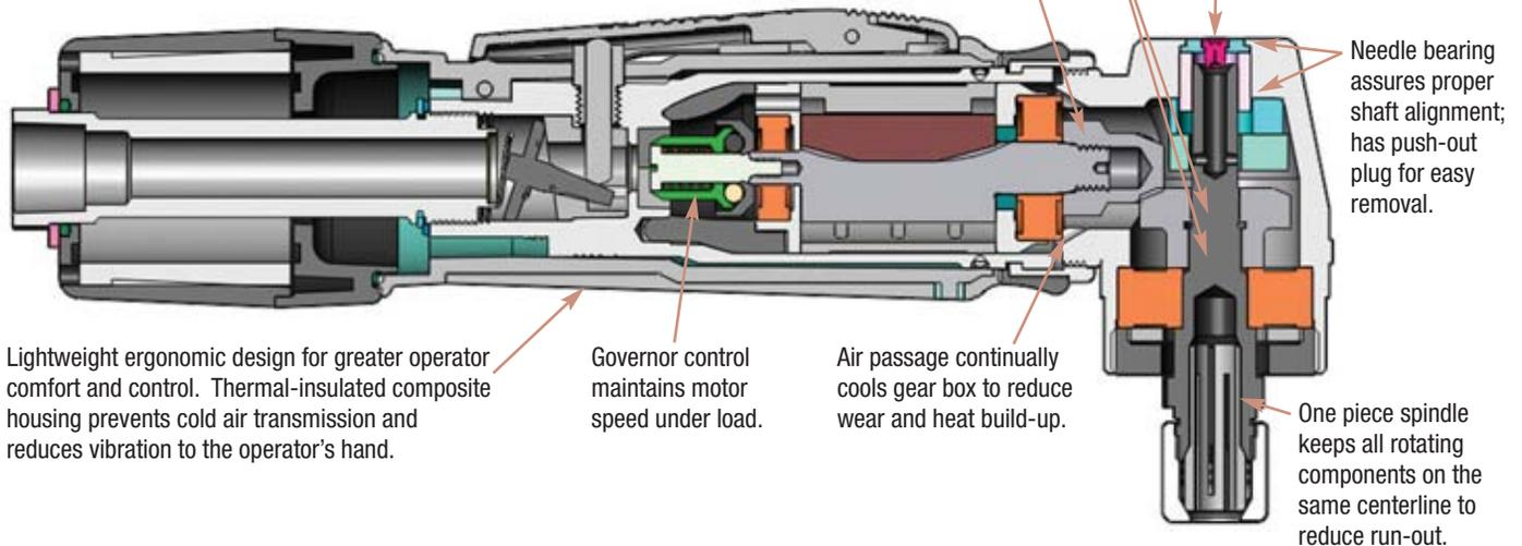
Lightweight ergonomic design for greater operator comfort and control. Thermal-insulated composite housing prevents cold air transmission and reduces vibration to the operator's hand.
