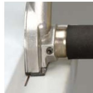
*Vacuum shroud cover may be used as a trim guide, for cutting as close as 5/32" (4 mm).*
