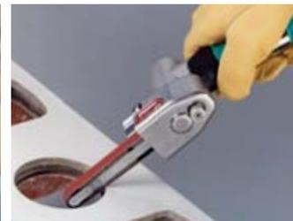
*Finish rough-cut edges quickly and efficiently.*
